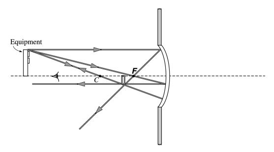
1 point each for any two correct principal rays (the three principal rays are shown above)
