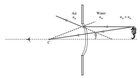
1 point each for any two correct rays (i.e. showing no refraction for normal incidence and refraction away form the normal for non-normal incidence)
