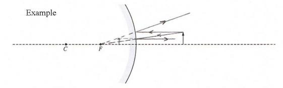
The ray diagram must contain at least two correct rays that show reflection and correctly show the image upright and smaller than the object, between the focal point and the mirror. The student must specifically indicate that his/her ray diagram is the justification to earn any points for it.
