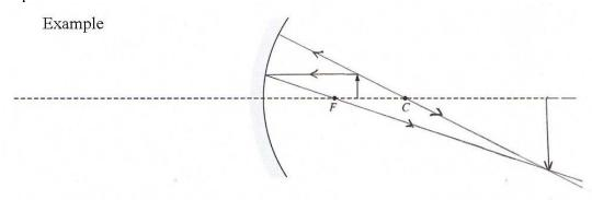
For a correct ray, correctly drawn (must reflect off mirror and must extend below principal axis)
