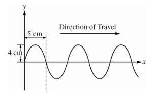
The figure above shows a transverse wave traveling to the right at a particular instant of time. The period of the wave is 0.2 s.
