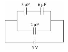
Three capacitors are connected to a 5 V source, as shown in the circuit diagram above.
